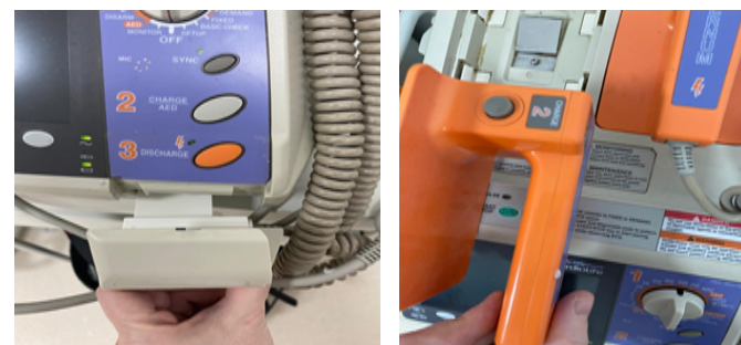
Figure 4. "charge" buttons on the defibrillator and spoons
