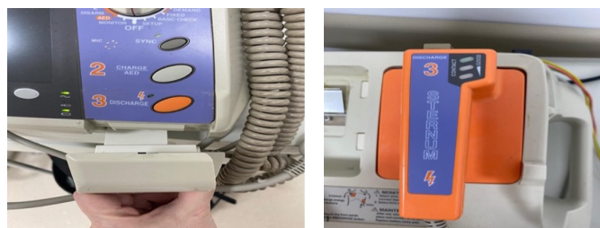
Figure 6. “Discharge” buttons on the defibrillator and spoons
