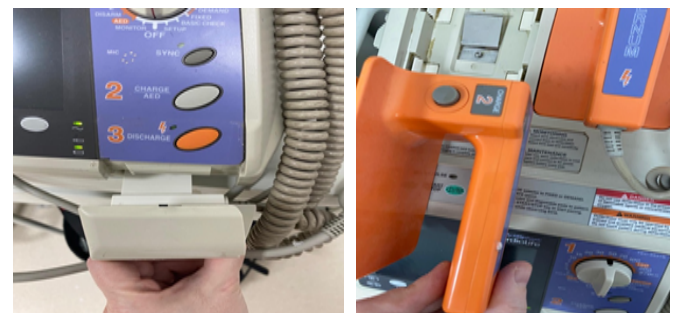
Figure 4. "charge" buttons on the defibrillator and spoons
