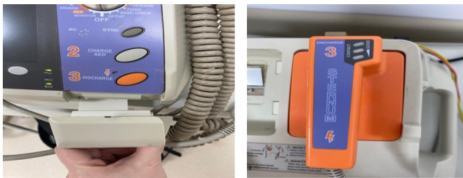
Figure 6. "discharge" buttons on the defibrillator and spoons
